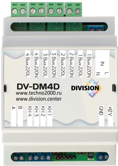
Picture 1. Appearance of DV-DM4D dimmer.
