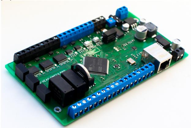
The device is made in a standard housing for installation on a DIN rail (9 DIN). The appearance of the DVC controller - HEAD PRO is shown in Figure 1.
